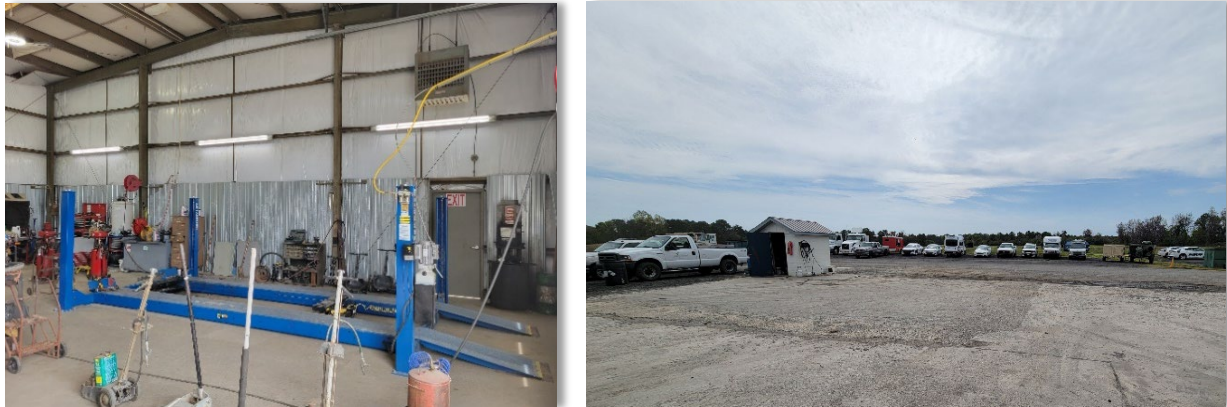
Figure 8. Four-post lift bay (left) and vehicle parking in the front of the garage (right)
